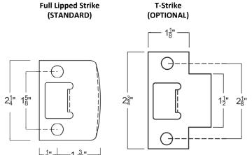
IMPORTANT: VERIFY TYPE OF STRIKE ORDERED BEFORE MORTISING JAMB STRIKE THICKNESS: 3/32" (INCLUDING THICKNESS OF DUSTBOX)
