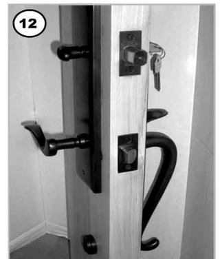
Check for alignment and operation, and tighten all fixings. On BZ trim fasten outside trim with the wood screws supplied.
